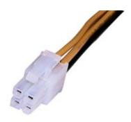
2. This is 20+4 pin connector; please only connect the 20-pin connector to the motherboard. Please **DO NOT** connect this 4-pin connector to the motherboard. (1 black, 1 yellow, 1 red and 1 orange wire)
